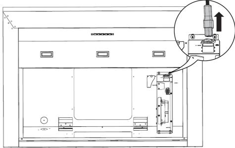
2. Remove the power cable from the hood and away from the strain relief. Place the strain relief back into the hole.
