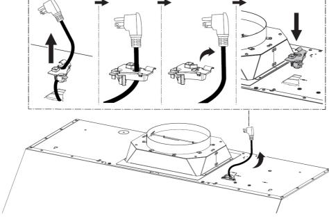
3. Attach the Wiring Box to the hood with 2 screws (G) in rear or top position.
