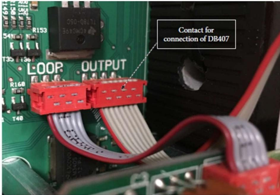
Please ensure that the EP104 is completely powered down before installation of the output card and that the desired outputs are wired in as per the below, and then power the EP104 back on.
