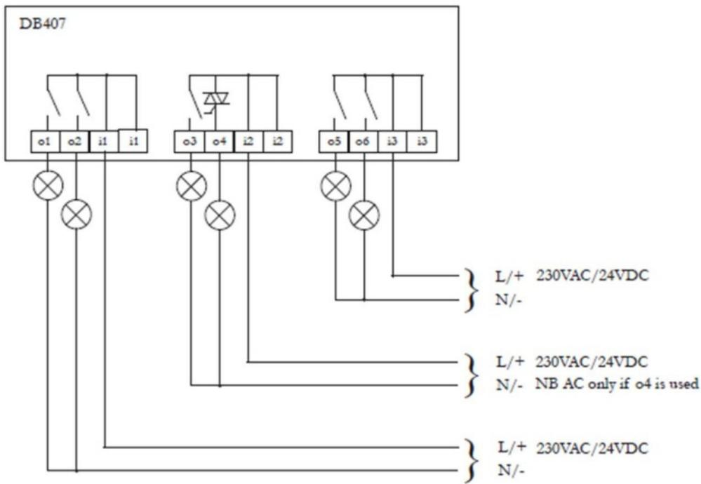
💡 If o4 is used for AC and o3 is to be used for DC, o3 can control an interposing relay
