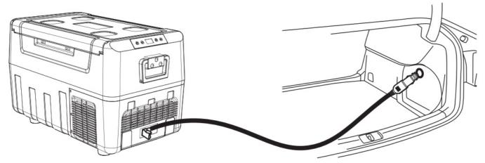
Connect the refrigerator to a portable power station and solar panel with the 1 00V-240V AC adapter.
