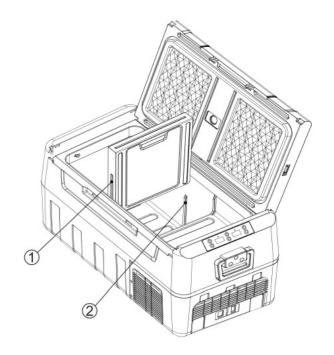
Under the working state, after inserting the divider, the panel displays the temperature of the two zones separately. When setting the temperature, the set temperature of the small zone must:\$ the set temperature of the large zone, for example: the small zone is set to -10°C (14°F), at this time, the large zone can only be set from -10°C (14°F) to 10°C (so°F).
