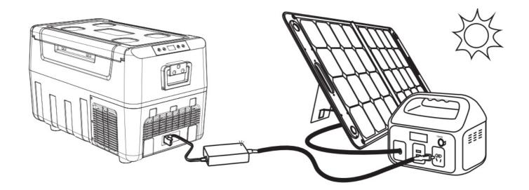
Connect the refrigerator to a portable power station and solar panel with the 12/24V DC cord.
