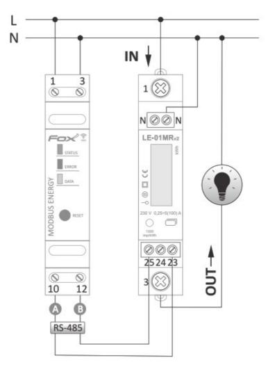
The connection scheme depends on the type of meter to be connected. Each time, the A-B communication outputs of the Modbus Energy integrator must be connected together with the A-B communication outputs of the energy meter. Example connection diagrams for all supported energy meters are available on the product page: <a href="https://www.fif.com.pl/fox/modbusenergy">www.fif.com.pl/fox/modbusenergy</a>.
