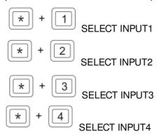
2. Keyboard switch (click 'Ctrl" twice, click No.1~4 the one you select) Ctrl+Ctrl + number(1~4) switch to 1~4 port you select. Ctrl+Ctrl + switch to previous port; Ctri+Ctri+ switch to next port.
