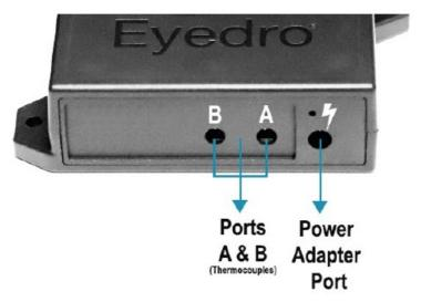
2. Connect thermocouple cables and power adapter to the Eyedro module.
