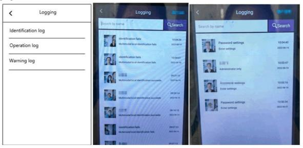
You can see the identification log, operation log and alarm log in logging. You can search by user's name to view the identification opening records and identification failure records in identification log. These records include the specific name, temperature, photo, identification result and time. Enter the operation log to view the entry setting record and time; enter the alarm log to view the monitoring video of the operation when the equipment is removed from the special brackets.
