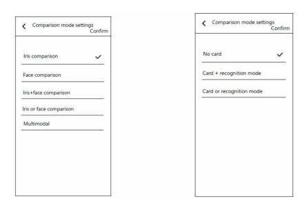
You can change the feature comparison modes in the comparison mode settings. The feature comparison mode includes Iris comparison, face comparison, iris & face comparison, iris or face comparison, and multimodal comparison. After turning on the Card swiping switch, you can select the card verification mode. The card verification mode includes: no card, card + recognition mode, card or recognition mode, and the comparison mode above can be changed according to user requirements.
