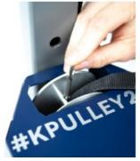
4. Cut off the damaged belt. Harden the edge with a lighter.
