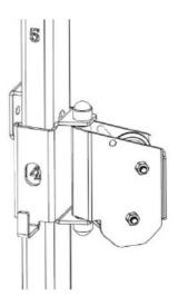
You can set the height the belt should come out from the kPulley using the numbers on the beam as a guide. Pull the knob to release the lock. Hold the sliding part in place and adjust the height, let go of the knob and let it click-in to lock the position.
