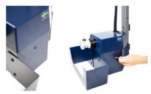
2. Hang the shaft cover on the height adjustment pulley hook.
