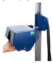
3. Unwind all of the belt from the shaft and use the 3 mm hex key to push the belt through the shaft and remove the lock pin.
