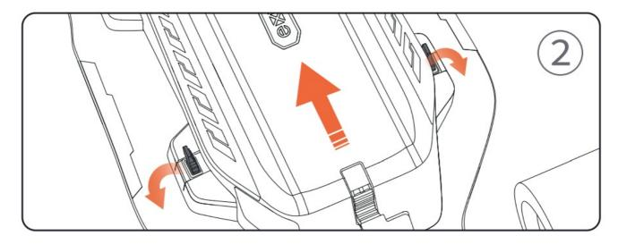
3. Lift the battery connector and push the battery in. Connect the power connector and make sure both locks are well fasten.
