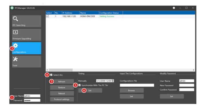
It's necessary to set the date and time no matter whether it's synchronized with the PC time or manually set, or else the below recording won't be valid and searched.
