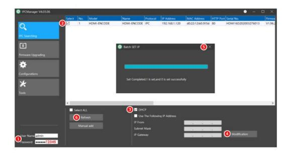
please ensure the encoder and your PC are on the same network segment if it's connected to the same router. That's why it's recommended to use DHCP to obtain IP address to make it for sure.
