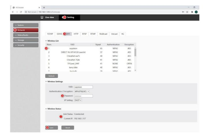
It's necessary to plug out the ethernet cable and power off the encoder to reboot it to make WiFi valid.
