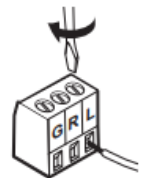
Figure 15. Connecting the PVT RGB D or PVT RGB D Plus to the PoleVault switcher
