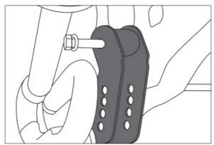
5. Attach the upper and lower control arms to the brackets and the vehicle body, as shown in the diagram.
