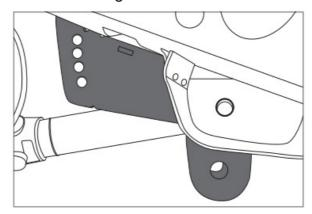
4. Connect the bushing end of the upper and lower control arm to the frame. Do not connect the ball joints to the steering joints yet.
