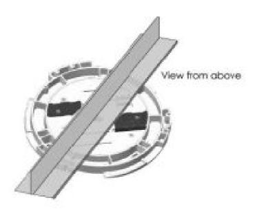
2 Rotate the bracket so that the flanges hook over the edges of the rall.
