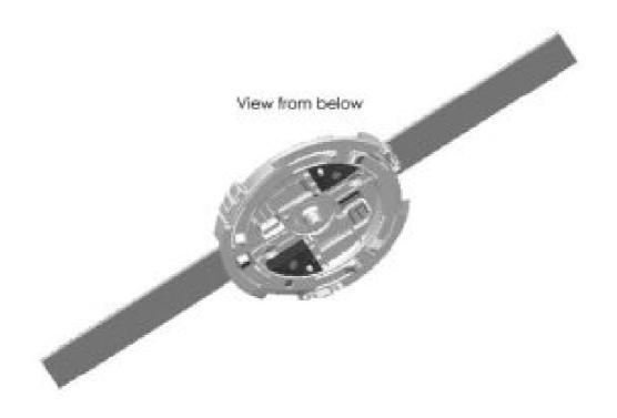
Once the bracket is secure, you can install the AP by aligning the red dot on the bracket with the red dot on the bottom of the AP. Keeping the dots aligned, raise the AP up until the bracket fits into the circular depression in the bottom of the AP. When the AP is firmly seated, rotate it clockwise until it clicks in to place. The process is identical for both models.
