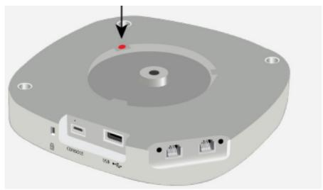
5. Rotate the AP clockwise until it clicks into place on the brackets
