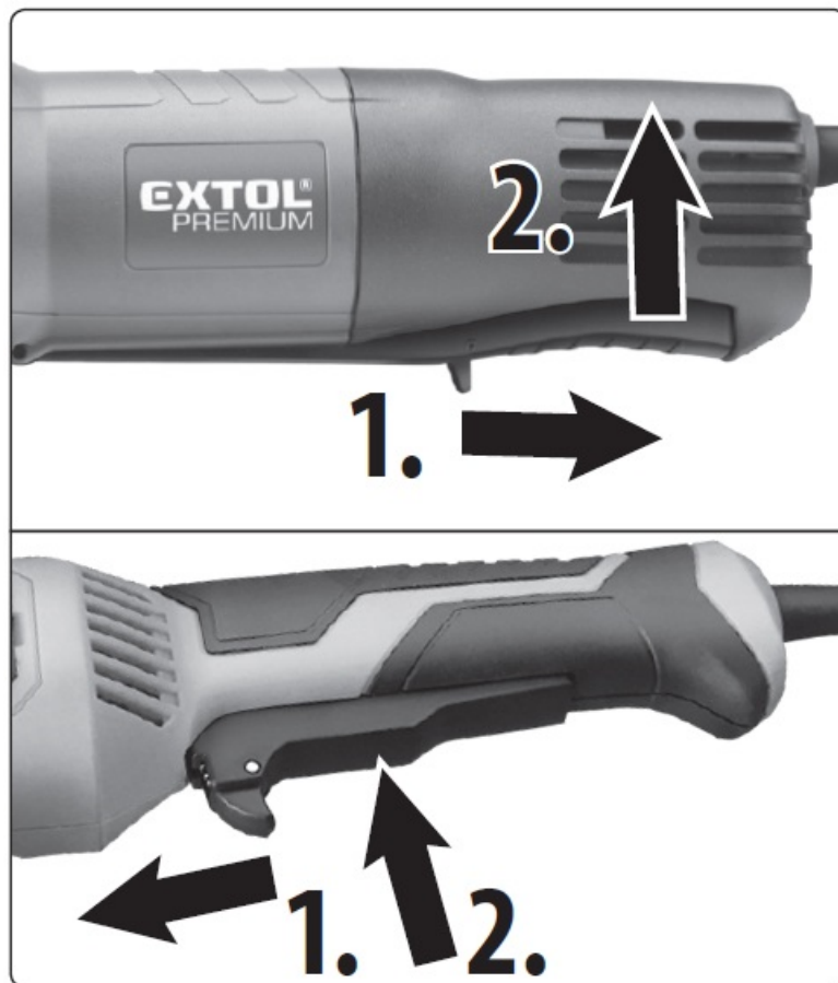
Fig.15; step 1. unlocking, step 2. starting
