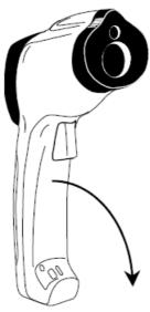
When the battery symbol appears in the display, replace the meter's 9V battery. The battery compartment is located behind the panel that surrounds the meter's trigger. The panel can be pried open near the trigger and folded down as shown in the diagram. Replace the 9V battery and close the battery compartment cover.
