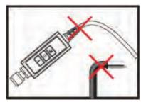
• Do not coil the probe to a diameter greater than 6 inches (15 cm) in use or when storing.
