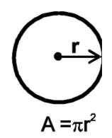
CFM (ft3/min) = Air Velocity (ft/min) x Area (ft2) CMM (m3/min) = Air Velocity (m/sec) x Area (m2) x 60
