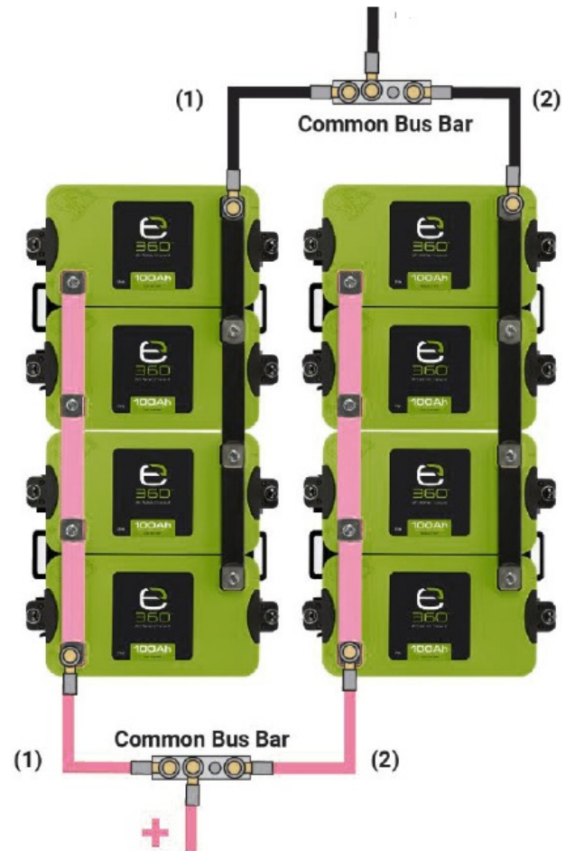
12 V 800 Ah 8 Batteries
