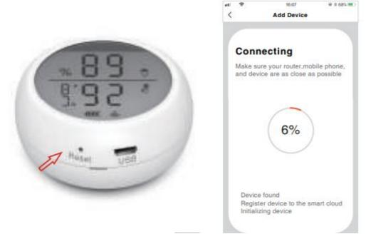
5. Under the automatic network configuration mode, press and hold the reset button with the Pin for 5 seconds to slow down flash of the indicator light as entering the manual network configuration mode. Choose the compatibility mode of APP and enter "WiFi password" according to the prompt and connect to network "Smart\_XXXX" to add device.
