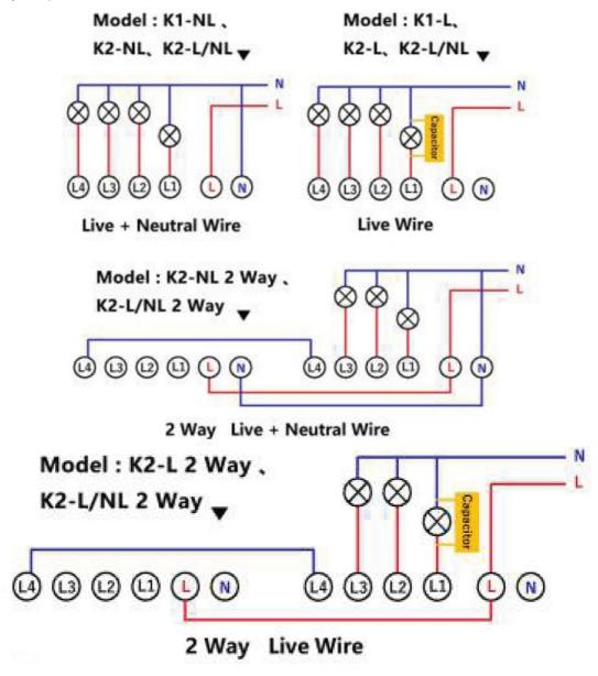
Without neutral wire is installed, The yellow Capacitor components must be distributed in parallel to Land N of the lamp holder connected in L 1 position (As shown in the wiring diagram)
