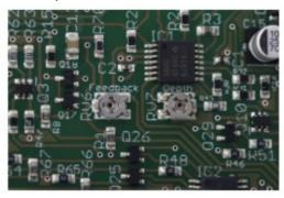
"RV6", marked "Feedback", scales the depth of the feedback control. It is factory-trimmed so that the feedback control turned fully clockwise doesn't quite send the module into selfoscillation. "RV7", marked "Depth", adjusts the relative levels of the original and phase-shifted signals. It is trimmed to maximise the depth of the nulls in the frequency response.
