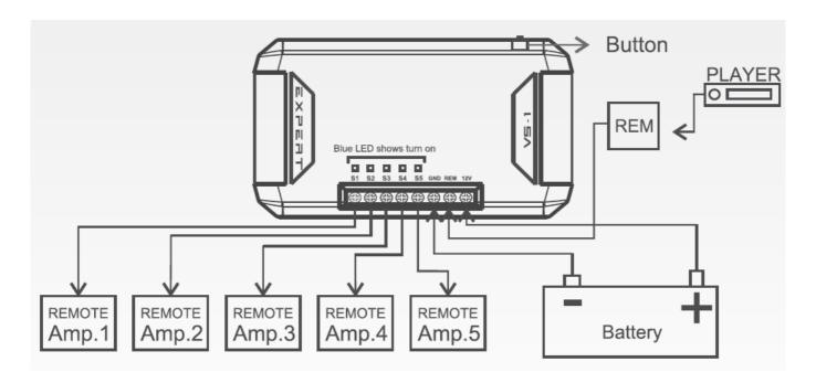
Use the remote from Player to turn on VS-1. Outputs S1, S2, S3, S4 and S5 can be connected to amplifiers.
