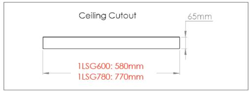
**WARNING:** Check for clearance of ceiling framing.
