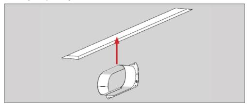
3. Connect the duct to the spigot using duct tape and cable tie
