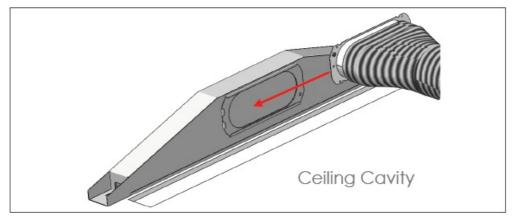
6. Secure the spigot to the plenum with an M5 screw
