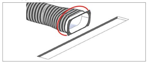
4. Connect the duct to the spigot using duct tape and cable tie
