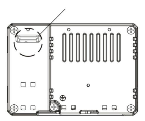
These devices are equipped with rechargeable Lithium battery, not user-replaceable.
