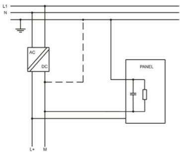
Ensure that the power supply has enough power capacity for the operation of the equipment. **CONNECTIONS**
