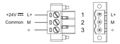
DC Power Connector, Female – R/C Terminal Blocks (XCFR2), manufactured by Weidmuller Inc., Cat. No. BLZ 5.08, torque 4.5 lb-in 3 conductor 1,5mmq wire size minimum, minimum temperature conductor rating 105°C.
