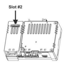
Slot#2 is available only if plugin module has the "bus extension connector". Each slot carries two communication channels:
