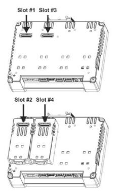
Slot#2 and Slot#4 are available only if plugin module has the "bus extension connector".
