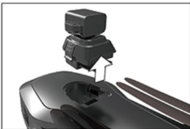
1. Remove the obstacle avoidance equipment as shown in the figure.
