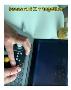
Please hold down A, X, B, Y together to swap the buttons' bindings with the placement typical of Xbox controllers
