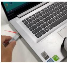
the bluetooth dongle is plugged into the PC.
