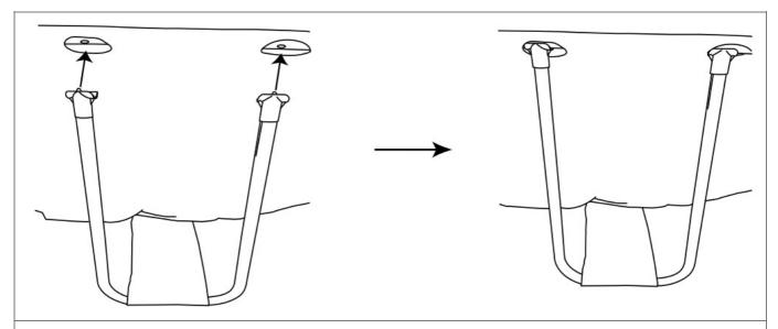
Find the one side holes on the horizontal beam. Place and lock the T-joints into the holes. Ensure they are fully connected
