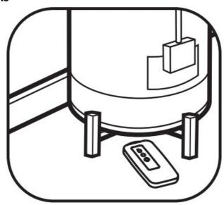
Locating a Water Sensor near the washing machine or its inlet valves is a good idea. Other locations can be under your water heater or near the sump pump in a basement.
