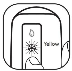
The Water Sensor has three built in commands. Step One – press and hold the button, the blue DROPLET will flash rapidly, then the yellow light will begin to flash. Step Two – Release on:
