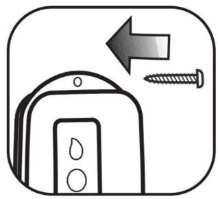
The mounting screw is included to allow for wall mounting. In certain situations, a user might prefer mounting the sensor on a vertical surface, above the floor, or in a sump.
