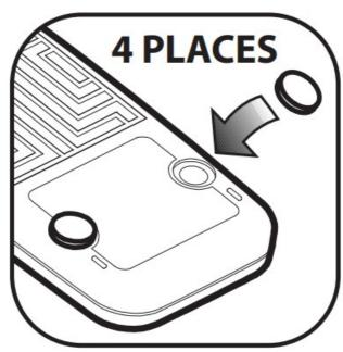
The rubber feet are designed to prevent the Water Sensor from sliding on the surface, yet to allow for easy cleaning under the unit. Just peel and stick the feet onto the sensor.
