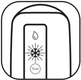
The blue SNOWFLAKE will flash blue when the surrounding temperature has fallen to 40°F or below. There will also be an audible warning tone. The Comm Link will send a text message.
