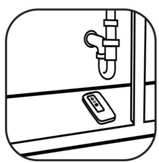
Excellent locations for Water Sensors are under sinks and dishwashers. Be sure that the placement surface is clear and will allow for a flow of water to reach the sensor.
