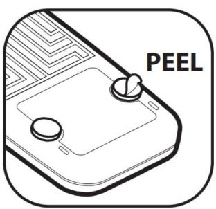
The 2-sided adhesive feet are included to create a more durable anti-sliding installation. Use of these feet prevents all movement of the device. Just peel the feet off the liner, stick to the unit, then peel off the secondary liner. Press the unit firmly to the floor/surface.
