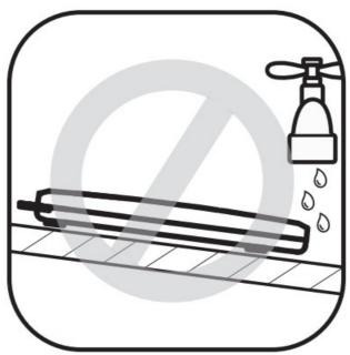
The Water Sensor must be placed in such a way as to ensure that water will move TOWARDS the sensor. This is often the lowest spot on a surface. The water must be free to flow, not be absorbed into the ground.
