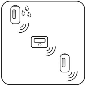
After installation, test all devices for Comm Link reception. Simply press and release the test button of a unit, then check your OmniShield App or text messages.
