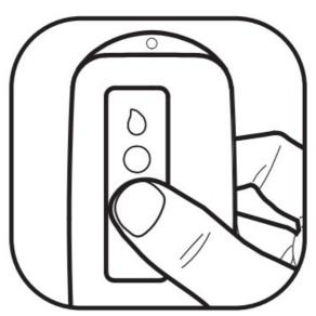
To activate your Water Sensor, simultaneously press the button on the front face while touching the gold/red sensor on the back. The Water Sensor will turn on and display a flashing blue light. After the sensor has bound with your Comm Link, the light will go out.
