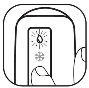
A single button press will test the Water Sensor. The unit can also be tested by applying a dab of water directly on the active portion of the sensor. The Comm Link will send a text msg.
