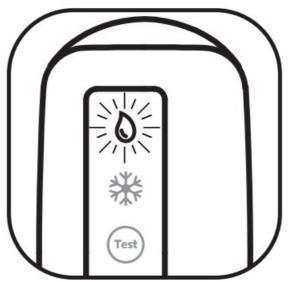
The blue water DROPLET will flash blue when water has been detected. This will be accompanied by an audible warning tone. A text message will be sent by the Comm Link.
