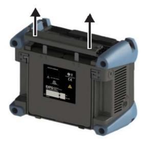
5. Use the markings on the back panel to locate the battery that you want to replace, and then pull on the battery's tab to free it from its socket.
