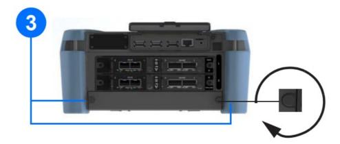
4. Remove the battery compartment door.
