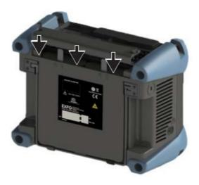
9. Turn the two retaining screws clockwise until they are tightened.
