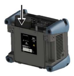
8. Place the battery compartment door on the unit so that it is flush with the top and back of the unit. If necessary, slightly move the battery compartment door until alignment is correct.
