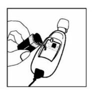
2. Depress the black release button and remove the cable while holding the release button down.
