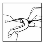
3. Orient the cable plug properly for a proper fit into the receptacle hole and install the replacement cable.
