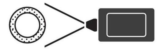
Contact the nosepiece to the surface and the D-Series will display an accurate surface temperature.
