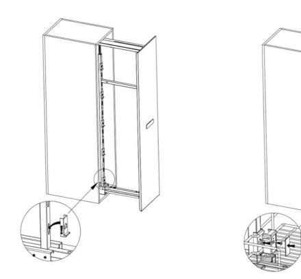
4. The graph shows the finished condition, and to ensure that the baskets are well installed, please press the edge of baskets to make sure that the edges are attached to the plastics fixed point (H).
