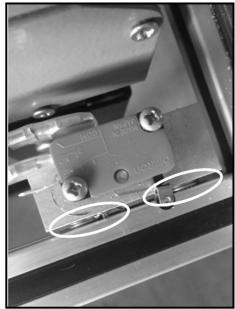
Connect the wires from the cut-off switch on the enclosure in place of ones supplied with the basic unit. **Note:** Take care during installation that the main power cable does not to obstruct the rear door.
