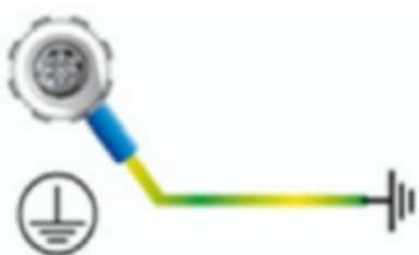
Figure 1: Socket-outlet protective earthing connection
