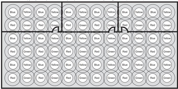
**Note:** Should you need to order additional detectors for an existing installation and need specific colour-coded detectors, please add the following suffixes to the part number: Y = Yellow, B= Blue, G= Green, R = Red. (There is normally no need to specify the colour codes as orders are dispatched with a suitable colour-code mix.)
