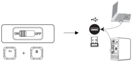
**4G mode:** Insert a dedicated receiver that has been paired with the code, and turn the switch to the "ON" position, FN+B enables 2.4G mode, and the keyboard can be used normally.
