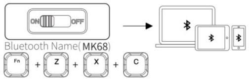
**Bluetooth mode:** Turn the switch to the "**ON**" position, There are three Bluetooth channels in total: **FN+Z:** Bluetooth 1 **FN+X:** Bluetooth 2 **FN+C:** Bluetooth 3. Turn on Bluetooth pairing on the device, and the keyboard can be used normally.
