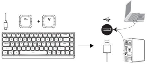
**Wired mode**: First, plug the connecting cable into the **TYPE-C** interface, and then connect the other end to the computer, **FN+V** enables wired mode, and the keyboard can be used normally.
