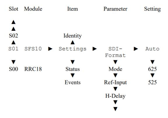
REMARK: Further information about Front Panel Control and Synapse Set Up Software can be obtained from the RRC18 and RRC04 operational manuals.
