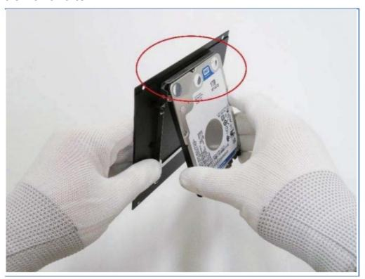
8. Align the hard drive with the bracket.
