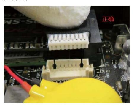
13. Insert the hard disk cable into the 9PIN interface of the motherboard. As shown in the photo. Connector upside down. please pay attention to the up and down orientation of the connector.
