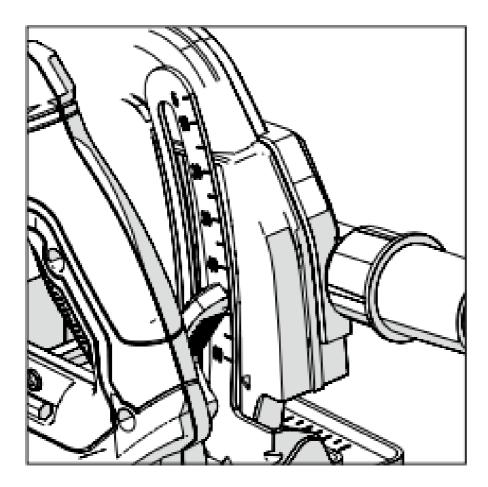
**Note:** Although the depth scale and index mark are very useful, enabling rapid depth setting, using them should always be regarded as a guide to the setting achieved. If a very precise depth of cut is required, then the blade setting should be checked with an engineers precision ruler (not supplied) or similar and adjusted accordingly
