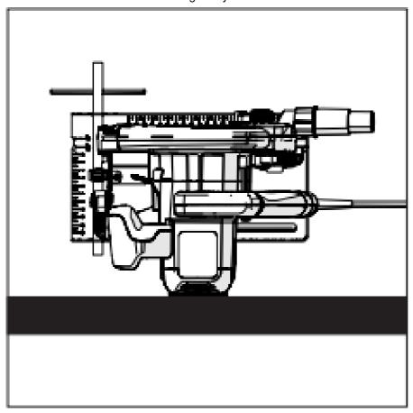
• Locate the machines arbor lock button (which is similarly positioned on all machines). Lock the machines arbor by operating the arbor lock button. (Fig. 3)
