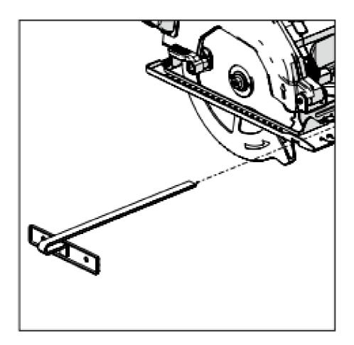
**Note:** The Parallel Edge Guide can be fitted on either side of the sole plate.
