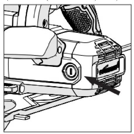
**Note:** Used but serviceable brushes can be replaced, but only as long as they are returned to the same position, and inserted the same way round as they were before being removed from the machine.
