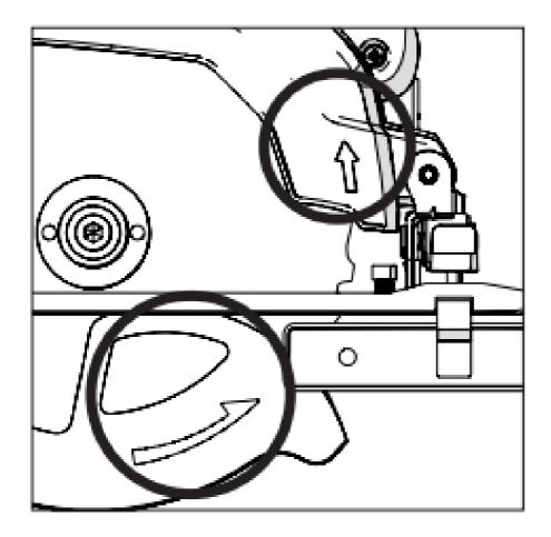
**Note:** The outer drive flange has a specially machined bore which incorporates two opposed 'flats.' (**Fig. 7**) These 'flats' engage with two complimentary 'flats' machined into the machines arbor shaft.
