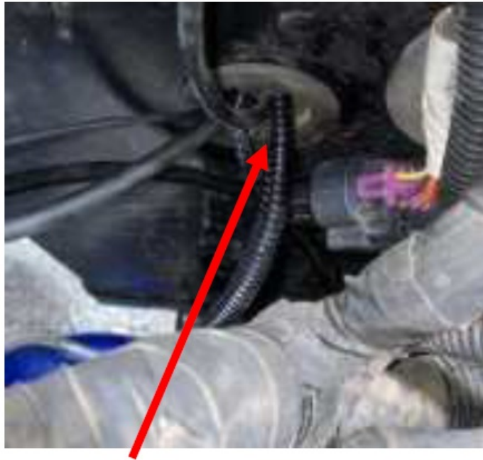
Figure 7, AFR Cable ran through the firewall into the cab.
