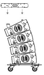
4. Unlock the bottom EVO88 element from the transport cart and proceed to suspend the system up to a comfortable position for next step.
