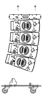
5. Lift the four top elements to a level where the next EVO88 elements in the transport cart naturally allaign the already set-up array and repeat the above steps.
