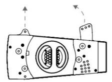
2. Position and lock the front and back links of the following element in the array using the spare pins stored in the dedicated hole labelled as Stow.
