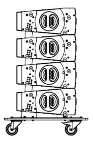
2. Set the proper internal spaly angles of the EVO88 elements while still on the transport cart for a more convenient, quicker setup operation.
