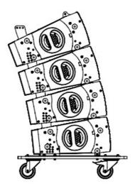
3. Fit the flying rigging frame RF-600 to the top element of EVO88 using the included locking pins.
