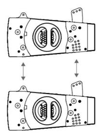
3. Finally lock the desired position with the dedicated pin stored in the Groundstack/Stow hole. Repeat the operation for the any other EVO88-M element in the system.
