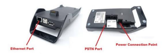
Once the Base and any additional cabling is connected, place the terminal in the charging base and allow the device to power up. This will take approximately 2 minutes. The Terminal will automatically pick-up the best mobile network available. If using an Ethernet connection, the terminal should obtain a valid IP address and connection automatically once connected to an Active Ethernet Port
