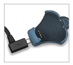
Line up the four gold pins on the bottom of the smart transmitter with the four gold pins on the charging cradle.
