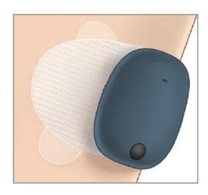
3. Check the connection between the smart transmitter and the sensor.
