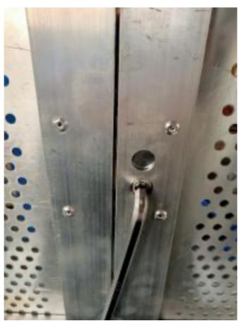
**Note:** Ensure the handrails line up where they should be, if not loosen up the bolts with the Allen key and the coffin latch and realign and tighten again.
