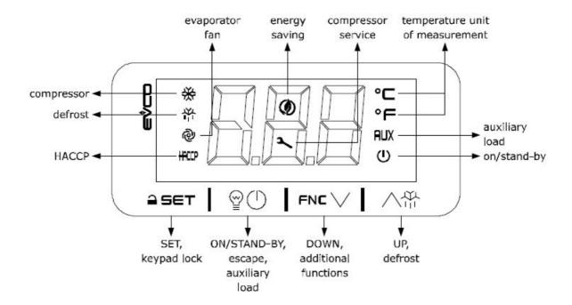
Switching the device on/off
