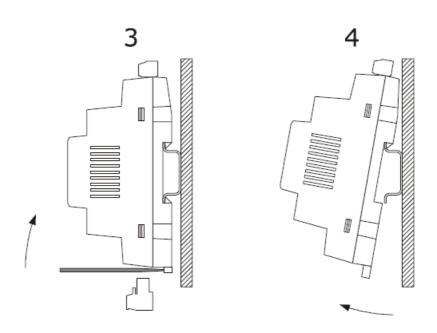
To install the devices again press the DIN rail clips to the end first.
