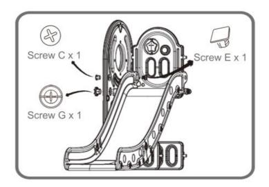
Attach the U-Shaped Panel, secure this side with 6pcs Screw C, 1 pc Screw G and 1 pc Square Screw E.
