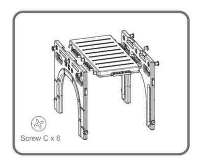
Install the 2 Security Fences on the Tunnel Panel.
